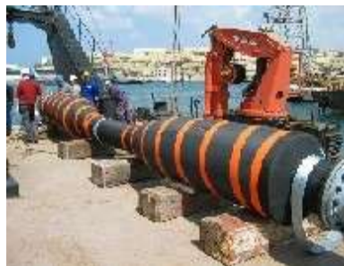
298 METER OFFLOADING HOSE ASSEMBLY
