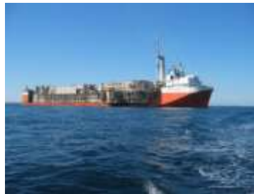
MIGHTY SERVANT 3 LOADED WITH 4 HULL STRIPS
